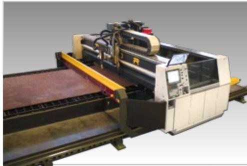
Front of the machine for thermal cutting
